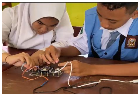
Image 2. Students assembled NodeMcu and TDS Sensor
